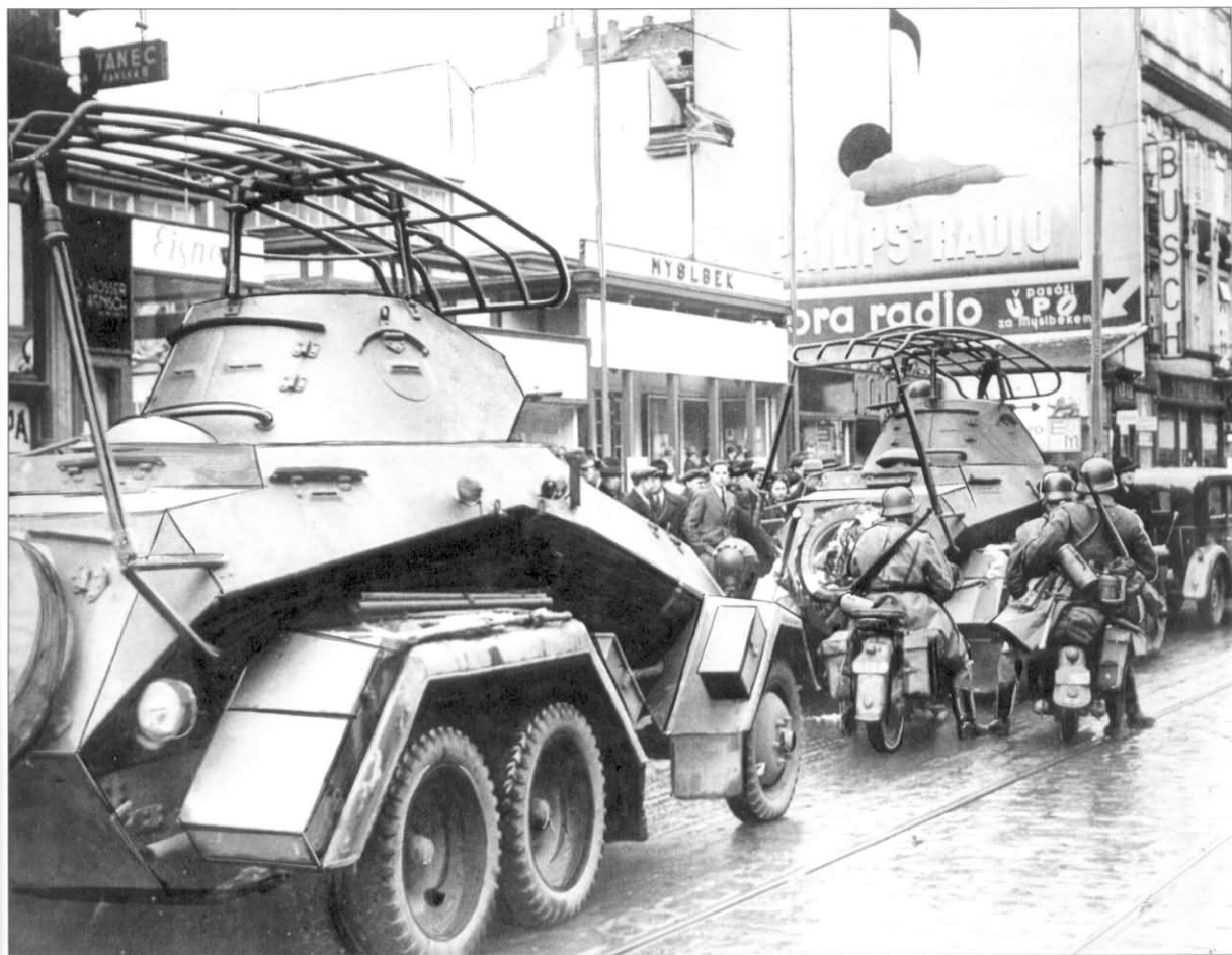
Reconnaissance troops of a Panzer-Division enter Prague, Czechoslovakia on March 15, 1939. Both vehicles seen here are schwere Panzerspähwagen (Fu) (Sd.Kfz.232) 6-Rad. The vehicle was equipped with a rear facing steering wheel and the visors on the rear allowed the car to be driven in reverse should enemy forces be encountered.
