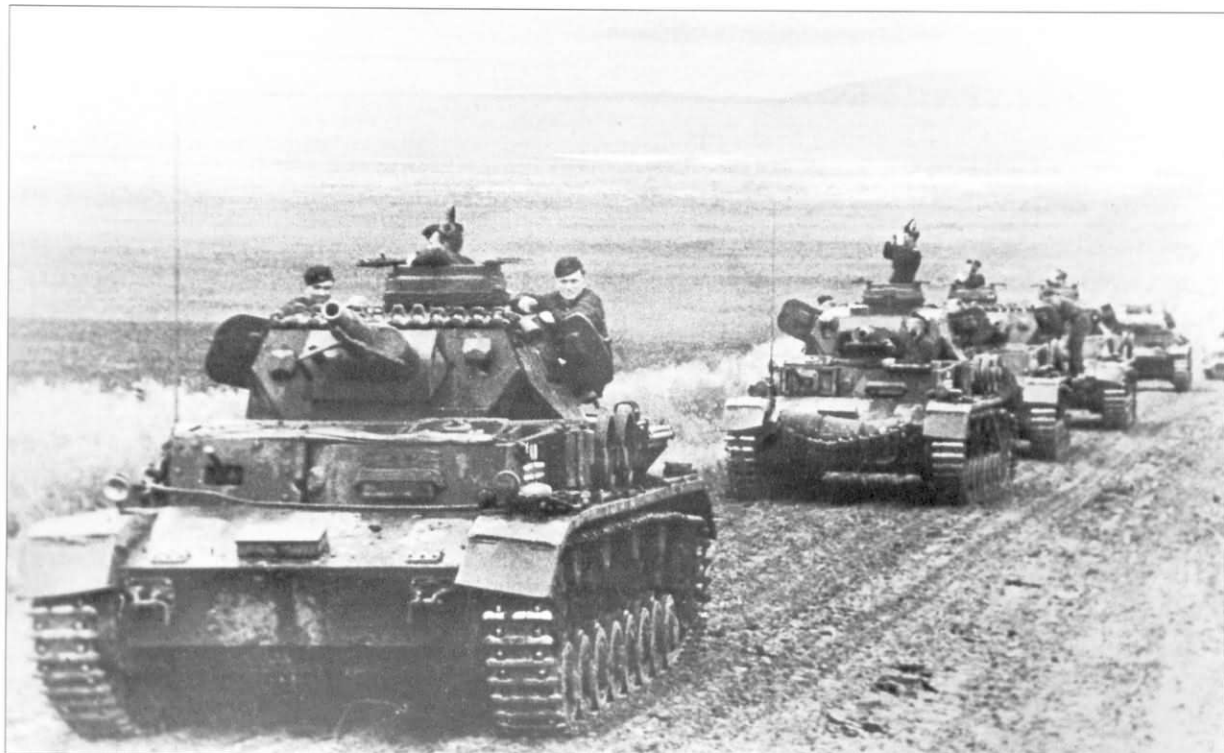
A column of tanks and softskin vehicles led by a platoon of Pz.Kpfw.IV Ausf.E carrying the emblem of 9.Panzer-Division beside the driver's visor. At the time, the Pz.Kpfw.IV was the heaviest tank in the German arsenal. Compare these vehicles to the photo of the ones crossing the Danube into Bulgaria seen earlier in this book. Unusually, the spare roadwheels carried on the first vehicle are two single wheels and not pairs. Also, the second vehicle in line does not have the additional 30mm armor plate installed on the front of the hull although the mounting brackets for it have been.
