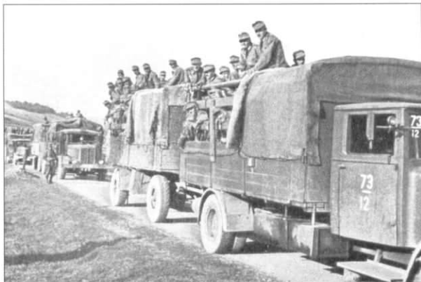
Lack of military transport in all the German divisions often forced commanders to use trucks borrowed from supply companies. Here, soldiers are transported in lorries towing trailers. The second vehicle is a Büssing NAG 6500 which is towing a 5-t trailer. The meaning of the numbers '73/12' on the first truck are unknown.
