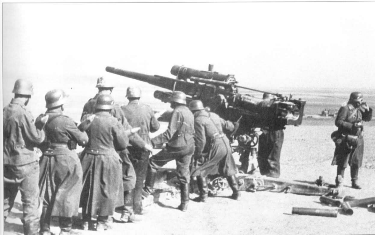
The gun crew queues up with rounds for their 8.8cm FlaK18 in northern France, late May 1940. Taken in the heat of battle, the gun is in full recoil and empty shell casings litter the ground around. The Pzgr.39 armor piercing round could penetrate 122mm of armor plate at a range of 1,000 meters, so no Matilda or KV crew was safe from it. The letter 'O' is painted in white on the recuperator housing.
