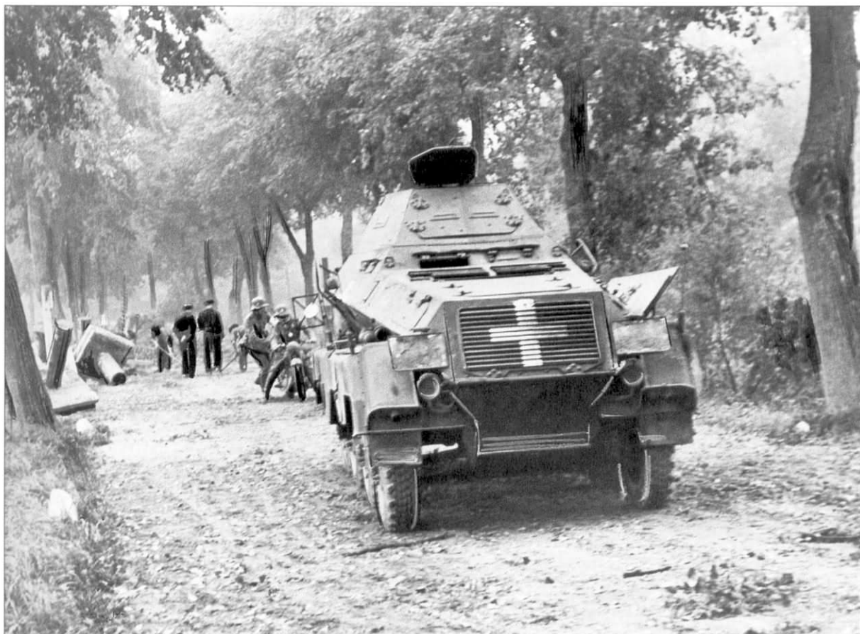
This retouched photograph shows German troops clearing away anti-tank obstacles placed across the road under the cover of a schwere Panzerspähwagen (Sd.Kfz.231) 8-Rad. It was the standard heavy armored car for the reconnaissance battalions in all of the Panzer-Divisions. The vehicle could be easily driven in two directions - forward and backward - because it was equipped with two sets of steering controls. The vehicle was long and heavy, so two sets of controls were necessary to allow the crew to retire in the opposite direction quickly if needed along narrow country roads. The only marking left by the censor is the white national cross painted on the rear of the car.
