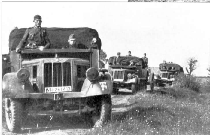
Three Sd.Kfz.11 half-track prime movers towing 10.5 cm IFH18 howitzers along a dirt road somewhere in France in 1940. The tactical sign on the mudguard of the first vehicle indicates they are attached to the first company of a towed artillery battalion. They are finished in overall dark gray with a heavy coat of dust. The Sd.Kfz.11 was used throughout the war to tow light and medium artillery and anti-tank guns.
