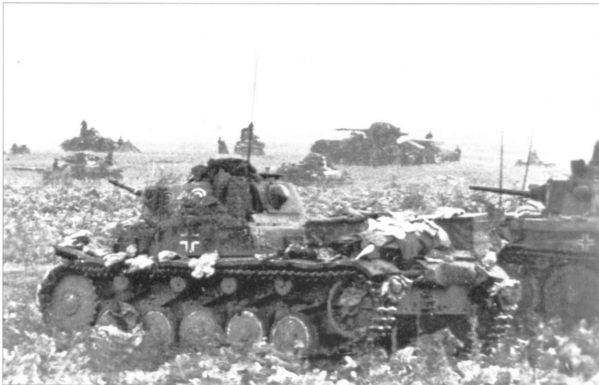
Regimental staff vehicles of a Panzer-Division halt in a field in Russia in late summer, 1941. Visible in the background are two 8.8cm FlaK18(SII) auf Zgw 12t (Sd.Kfz.8) and several other vehicles that have made some attempt at camouflaging themselves in the open ground. The Pz.Kpfw.II Ausf.A-C in the foreground has the tactical number 'R12' painted on the turret, possibly red with a white outline, while only the first letter of the tactical number can be seen on the Pz.Kpfw.38(t) behind it.
