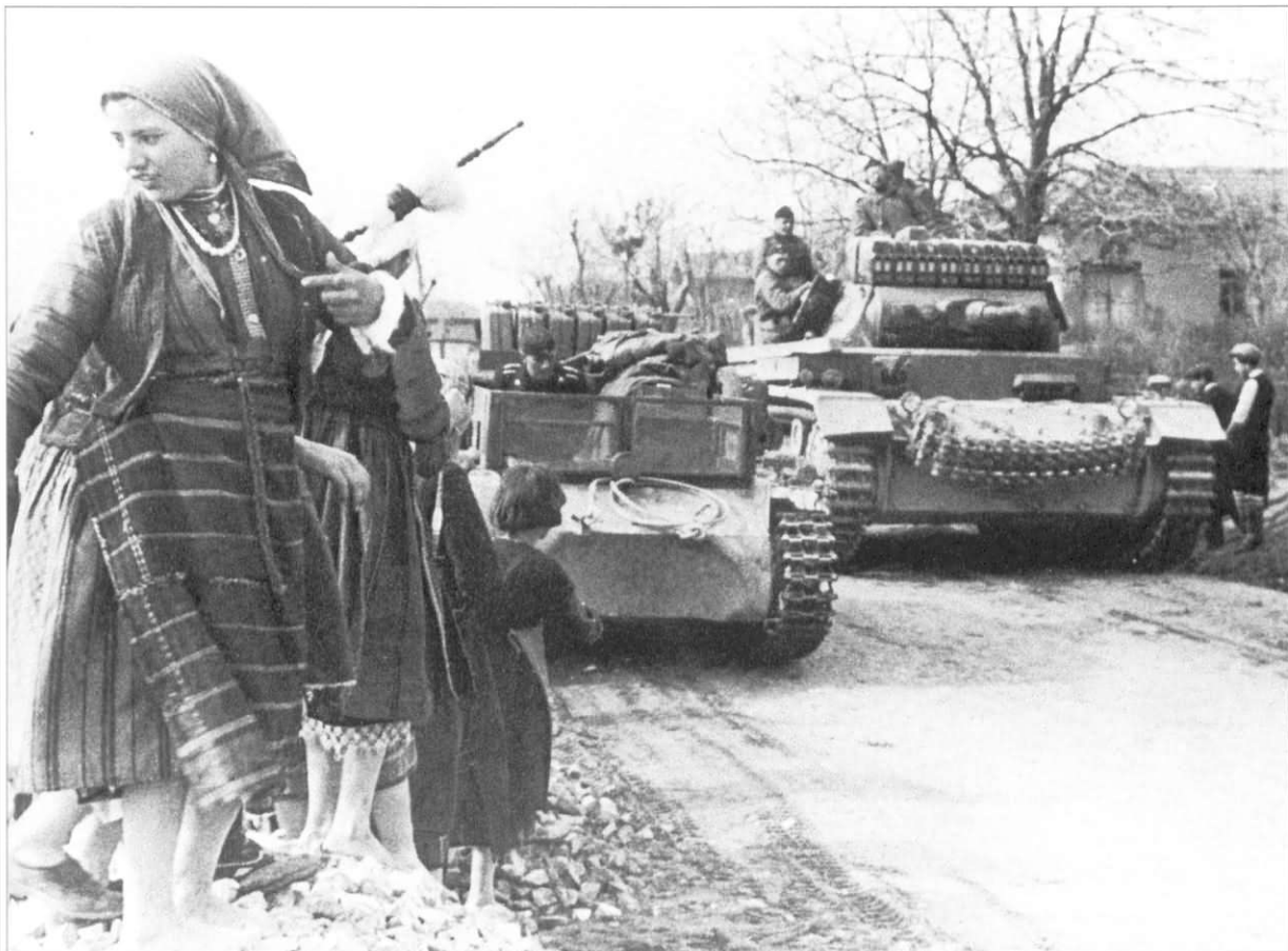
A Pz.Kpfw.III Ausf.G passing by another rare vehicle, an Instandsetzungskraftwagen I, an open, turretless Pz.Kpfw.I Ausf.B used as a repair and recovery vehicle. Unusually, this one features a glass windscreen. 164 of them were produced up to November 1938. They were used up to 1941 when they were found to be too small and after that served as training vehicles. The emblem of 9.Panzer-Division is just visible to the right of the driver's visor on the Pz.Kpfw.III. This photo was taken in Bulgaria in late March 1941.
