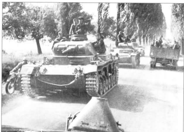
A Pz.Kpfw.III Ausf.F followed by a Pz.Kpfw.III Ausf.A-C and a Pz.Kpfw.I advance into France in May 1940. During the battle for France, the most numerous versions of the Pz.Kpfw.III were the Ausf.E and Ausf.F. Between December 1938 and July 1940, 531 vehicles of both types were manufactured. The cast air intakes on the glacis identify this one, otherwise they were very similar.
