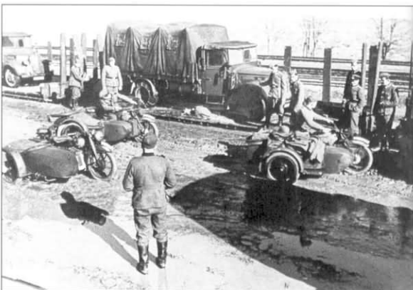
Another shot of vehicles being loaded onto trains. The two motorcycle combinations in the background are Zündapp KS600's. The one in front is a BMW R61 that has been fitted with an unusual sidecar. The two trucks are Ford G 917 T or G 997 T 3-ton lorries. The two types were identical externally, the only difference being the engine.
