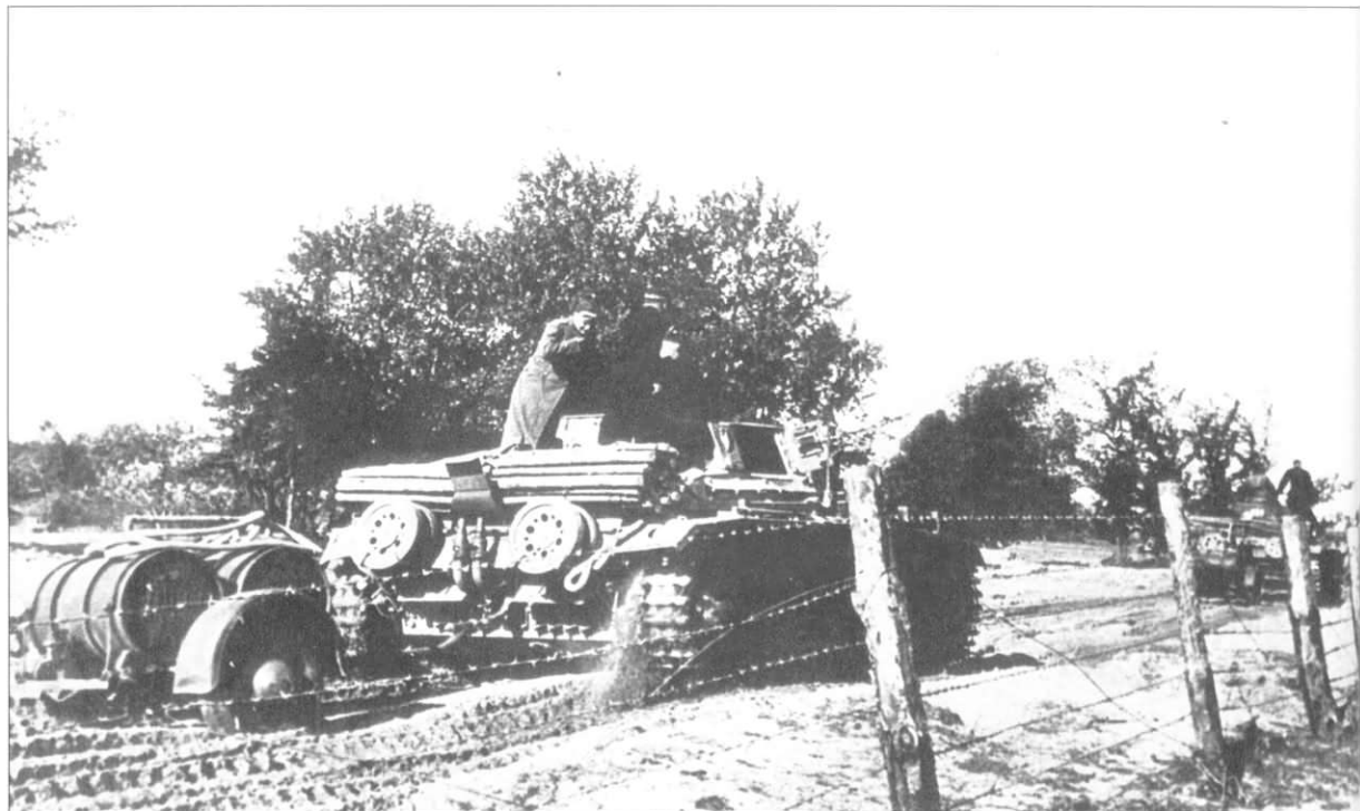
A Tauchpanzer III towing a special trailer carrying two 200 liter barrels of fuel, travels down a sandy road in the Soviet Union in late June 1941. From July to October 1940, 168 Tauchpanzer were converted from Pz.Kpfw.III Ausf.F, G and H in preparation for Operation 'Sea Lion', the invasion of Great Britain. When the operation was canceled, seventy-five percent of the vehicles were attached to 18.Panzer-Division with the remainder going to 4.Panzer-Division. The twin exhaust pipes with the specially designed backflow valves can be seen between the two spare roadwheels mounted on the rear plate.
