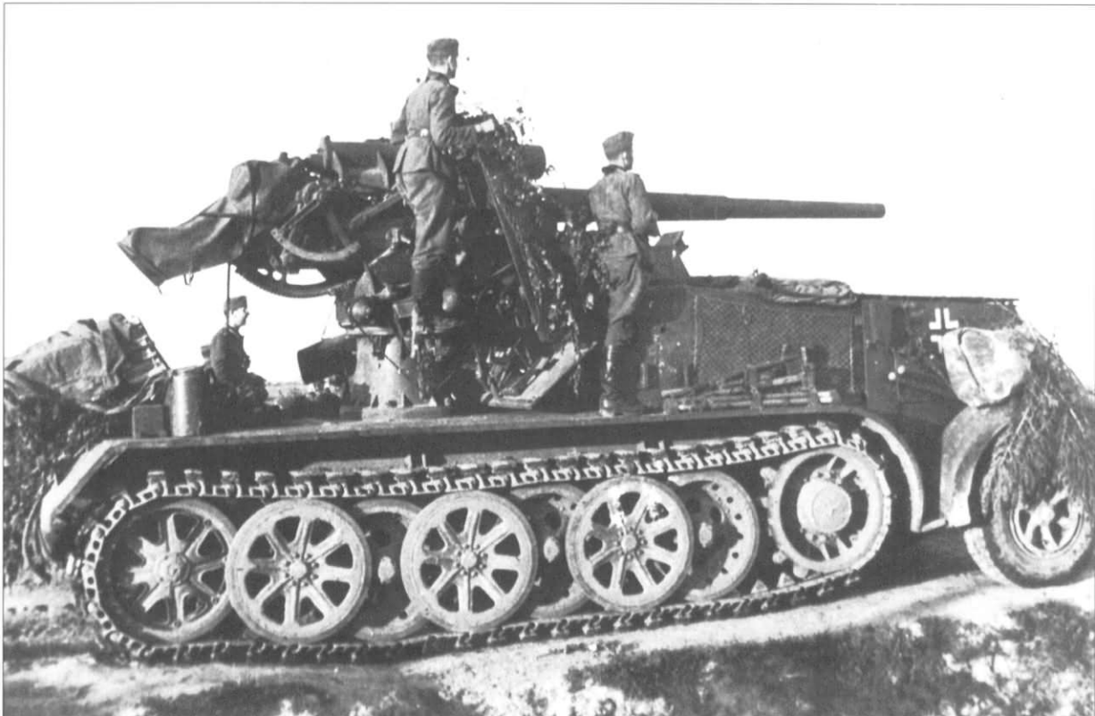
The 8.8cm FlaK18(Sfl) auf Zugkraftwagen 12t (Sd.Kfz.8) was used mainly as a heavy anti-tank vehicle in Poland and France. Only 25 were produced in 1939 and 1940 and they were issued to s.Pz.Jg.Abt.8. Subsequent versions were built on the 18t FAMO and were also intended for use in an anti-aircraft role.
