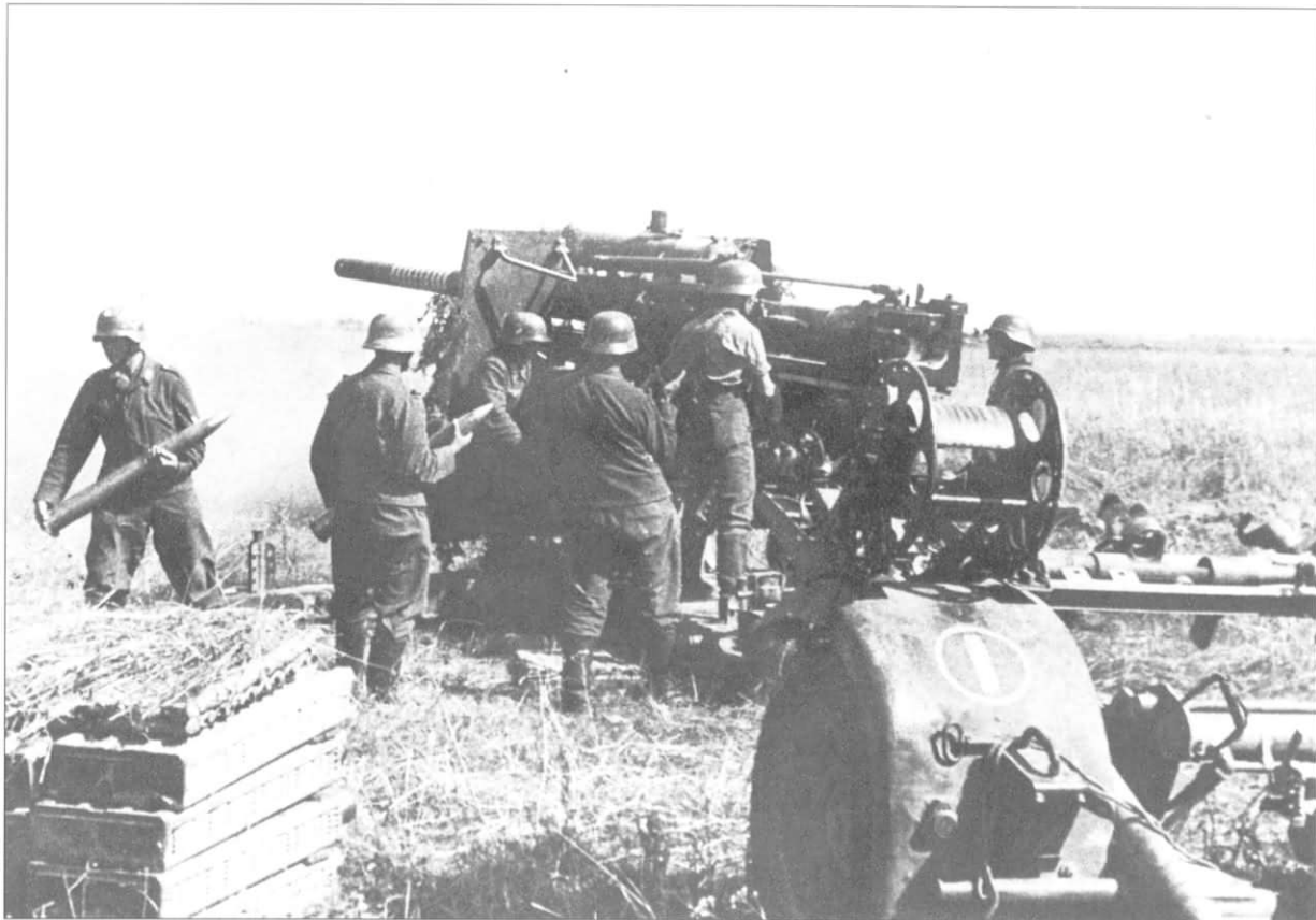
The most powerful anti-tank gun in use by the German Army was the 8.8cm FlaK18 and 36/37, shown here in full recoil. These guns were employed by Luftwaffe FlaK units and manned by Luftwaffe personnel. The crew of this gun are obviously experienced as indicated by the ten kill rings painted on the barrel. A tactical marking is painted on the mudguard of the trailer in the foreground.
