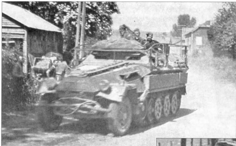
This Sd.Kfz.251/6 Ausf.A command half-track is fitted with an early style of frame antenna. The divisional emblem for one of the Panzer Divisions using a 'Y' is barely visible on the right mudguard.
