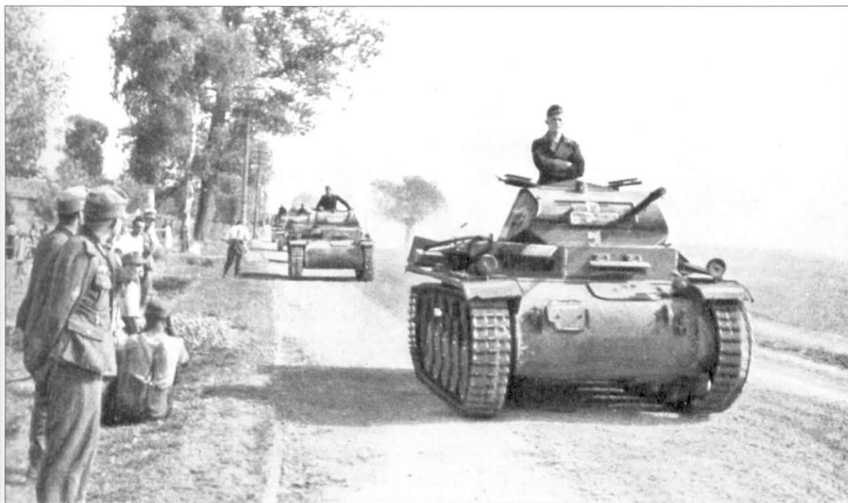
The battle over, these Pz.Kpfw.II Ausf.c-C head back to Germany for refitting and rest. After the defeat of Poland, the Pz.Kpfw.II was improved with additional 20mm armor plate on the front hull and turret. The white national cross that was painted on the front of this vehicle's turret has had mud or paint applied to make it less conspicuous to Polish anti-tank gunners.
