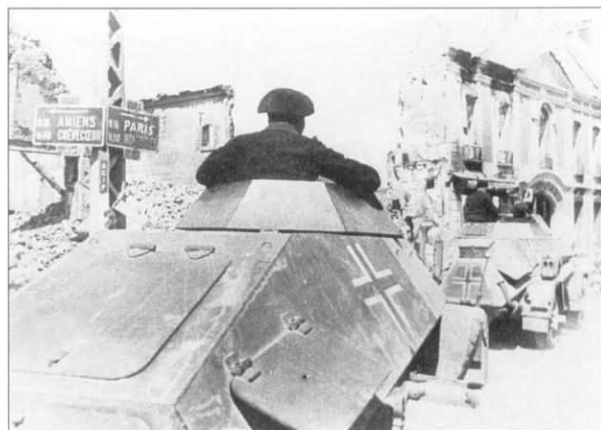
A pair of light armored cars make their way through a destroyed French town south of Amiens in June 1940. The leading vehicle is an Sd.Kfz. 222 while the one closest to the camera is an Sd.Kfz. 221. The Sd.Kfz. 221, armed with only one MG34 machine gun, was only produced up to May 1940 and so was obsolete by this time. Despite this weakness, it was utilized until 1942, when it was uparmed with the sPzB41 mounted in a modified fixed turret.
