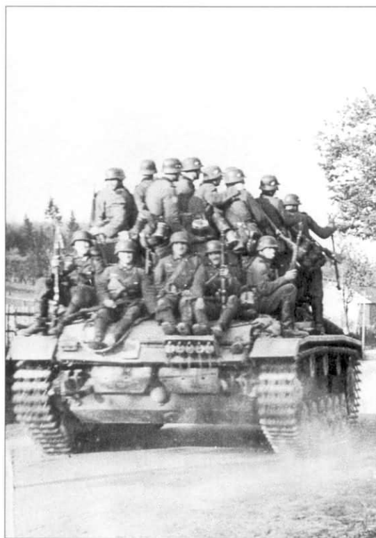
An infantry squad catches a ride on a Pz.Kpfw.III Ausf.F in France in early June 1940, a common practice throughout the war. Unusually, the rear Notek convoy light and tail light have been relocated from their normal position on the mudguard to the rear plate. The apparatus below the men's feet is a smoke candle rack that was operated from within the vehicle.
