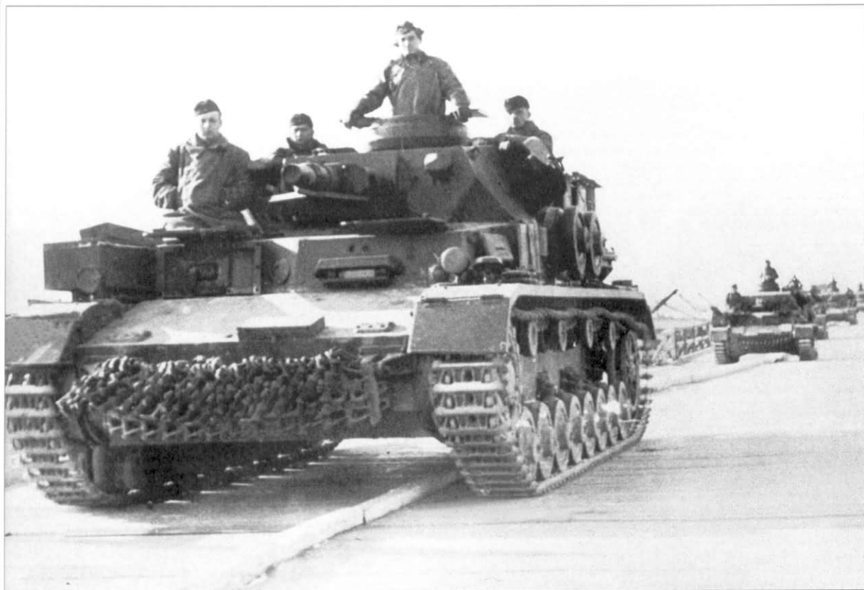
A column of Pz.Kpfw.IV Ausf.E from Pz.Rgt.33 of 9.Panzer-Division enter Bulgaria over the Danube bridge. Visible around the MG ball mount is the bracket for attaching the 30mm additional armor plate that was fitted to many of these vehicles. This crew have also suspended several rows of extra track links from the front tow hooks.
