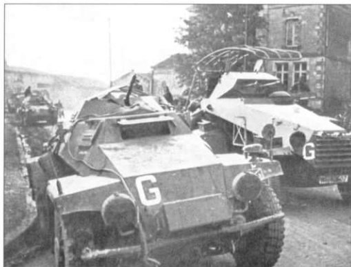
A schwere Panzerspähwagen (Sd.Kfz.232) (Fu) 6-Rad passes an Sd.Kfz.221 of 2.Panzer-Division in France in June 1940. Both vehicles carry the white letter 'G' for Guderian's XIX.Panzer-Korps, prominently displayed on the front. The Sd.Kfz.221 also has the tactical sign of a motorized reconnaissance unit with a '2' in the lower right corner, painted on the left mudguard. Beside that can be seen the two yellow dots representing 2.Panzer-Division. An unrecognizable inscription has been painted under the driver's side visor as well.
