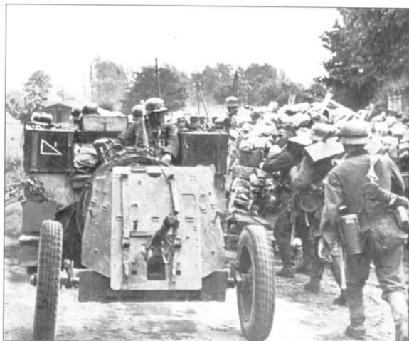
A Krupp Protze Kfz.69 towing a 3.7cm PaK35/36 past a barricade on a road in southern France in June 1940. This was not the only anti-tank gun used in the German divisions at this stage of the war as they also employed 4 companies of Czech-made 4.7cm anti-tank guns mounted on the Pz.Kpfw.I chassis. Nevertheless, the PaK35/36 was still the standard anti-tank gun in use although it was virtually obsolete by this time. The tactical sign painted on the back of the Krupp Protze indicates this unit belongs to the 1.Kompanie of an anti-tank battalion.
