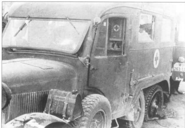
A German Steyr 640 Kfz.31 ambulance shot up by French troops in early June 1940. The Red Cross signs on sides and rear door are not very prominent which probably contributed to the mistaken identity. The front mudguard and rear door carry the emblem of Pz.Rgt.8 which at that time was one of the two Panzer-Regiments attached to 10.Panzer-Division.
